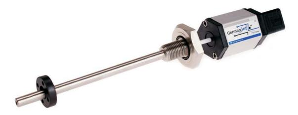
The sensor cartridge can be removed from the flange while still installed in the cylinder. This allows quick sensor cartridge replacement without the loss of hydraulic pressure.
