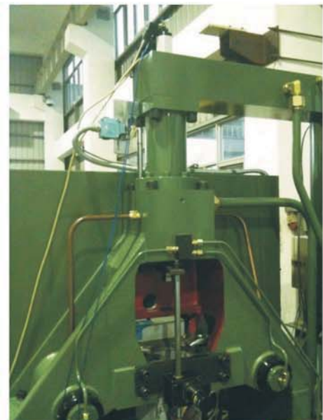
Hot chamber die-cast machine used Germanjet 17 series
