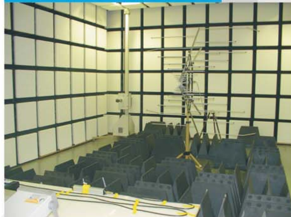
Radiated, radio-frequency, electromagnetic field immunity test
