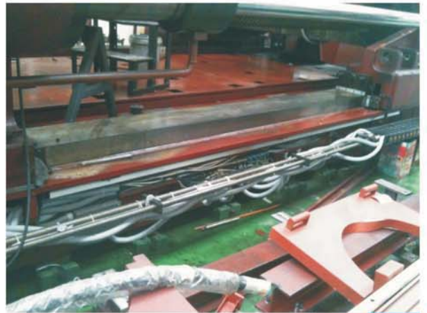
4000mm transducer installed at 6000 ton machine
