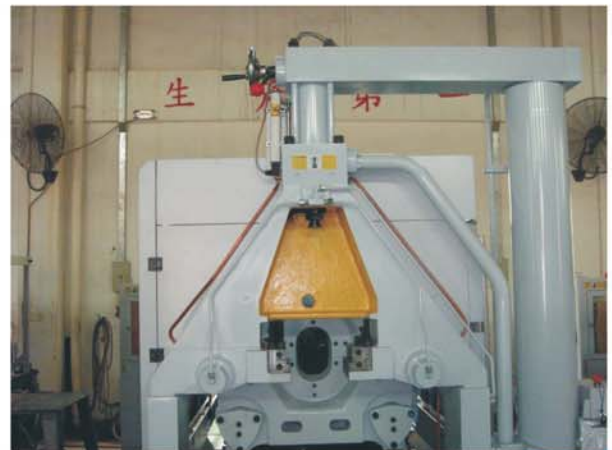
Hot chamber die-casting machine used Germanjet 18 series
