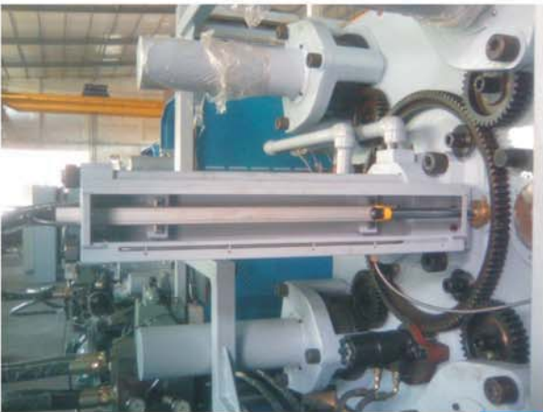
Mold closing at die-cast machine, injection speed at 10m/s
